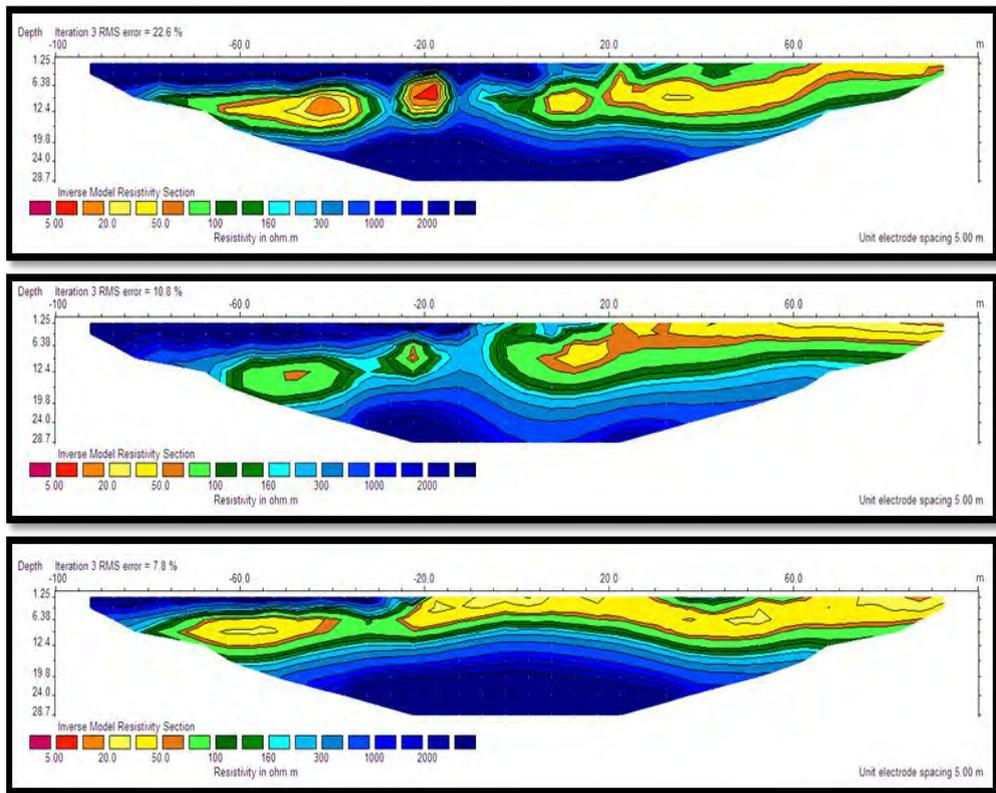
Figure 5: Inverse model of electrical resistivity section for profiles #4, #5 and #6 showing interpreted location of shallow limestone cavities and sinkhole.
