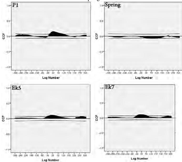
Figure 5. Cross-correlation function plot for representative wells of karst aquifers at southwest Izeh and Halaijan Spring
