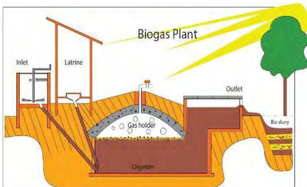
Fig. 12 Typical biogas plant for domestic wastewater
