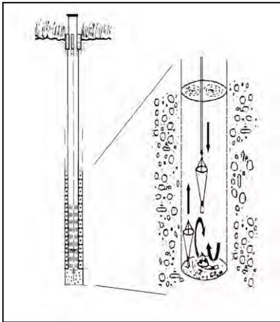
Figure 3: Modified Cvetkov net sampler, Fuchs (2007)
