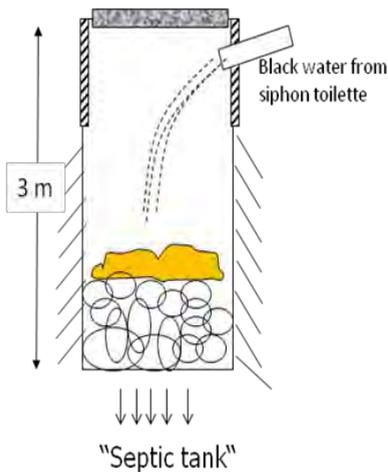
Figure 6. "Advanced infiltration pit"
