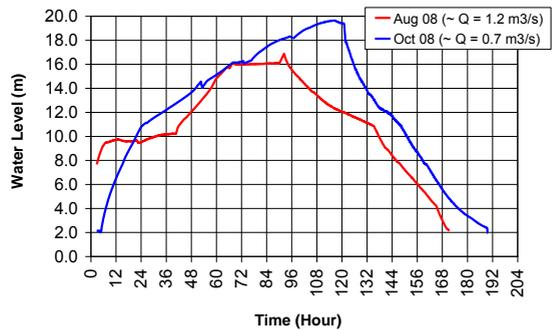
Fig. 12 Successful first storage and operational test in August 2008 (left) and storage curve (right), note: for monitoring purposes, the water level had constantly been held at several heights through partial opening of the controlling valves
