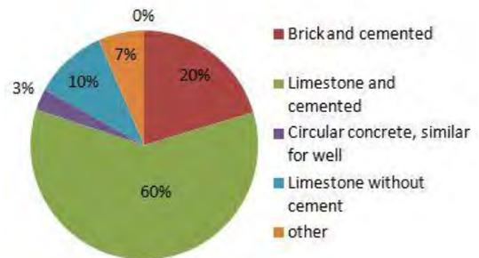
Figure 7. Material for septic tank construction
