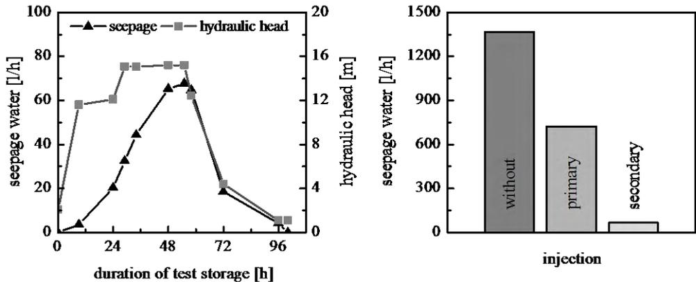
Figure 5. Exemplary graph illustrating the result of a test storage after the secondary injection measure (left) and comparison of seepage water amounts at different stages of the construction process (right)
