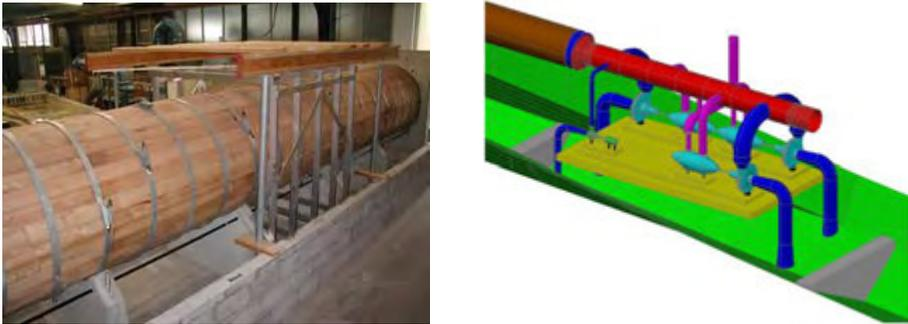
Fig. 13 Experimental investigation of wood-stave pipeline at KIT (left) and illustration of the planned underground hydropower plant in Gua Seropan (right)
