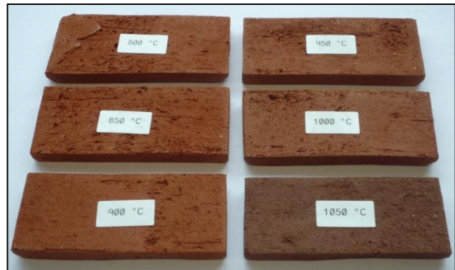
(b) Laboratory experiments: ceramic fired from local clay at varying temperatures
