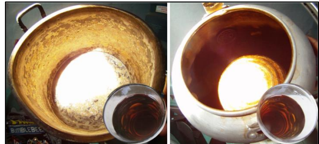
(b) Cooking pot and tea made from raw water (left) and filtered water (right)
