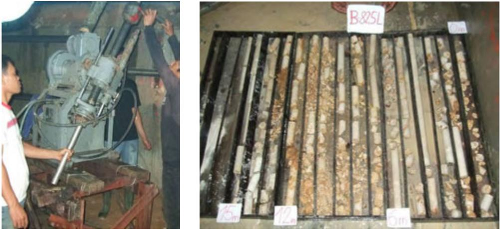
Figure 4. Drilling and injection equipment (left) and drilling cores providing detailed information on the karstification of the rock mass (right)
