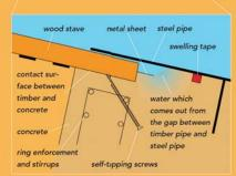
Wood stave pipelines can bebuilt above ground, supported by concrete saddles, or in a dtch that is subsequently filled in. To make termite activity more visible, the wood stave pipeline should be a minimum of 200 mm above ground and a termite shield arranged on each support.
